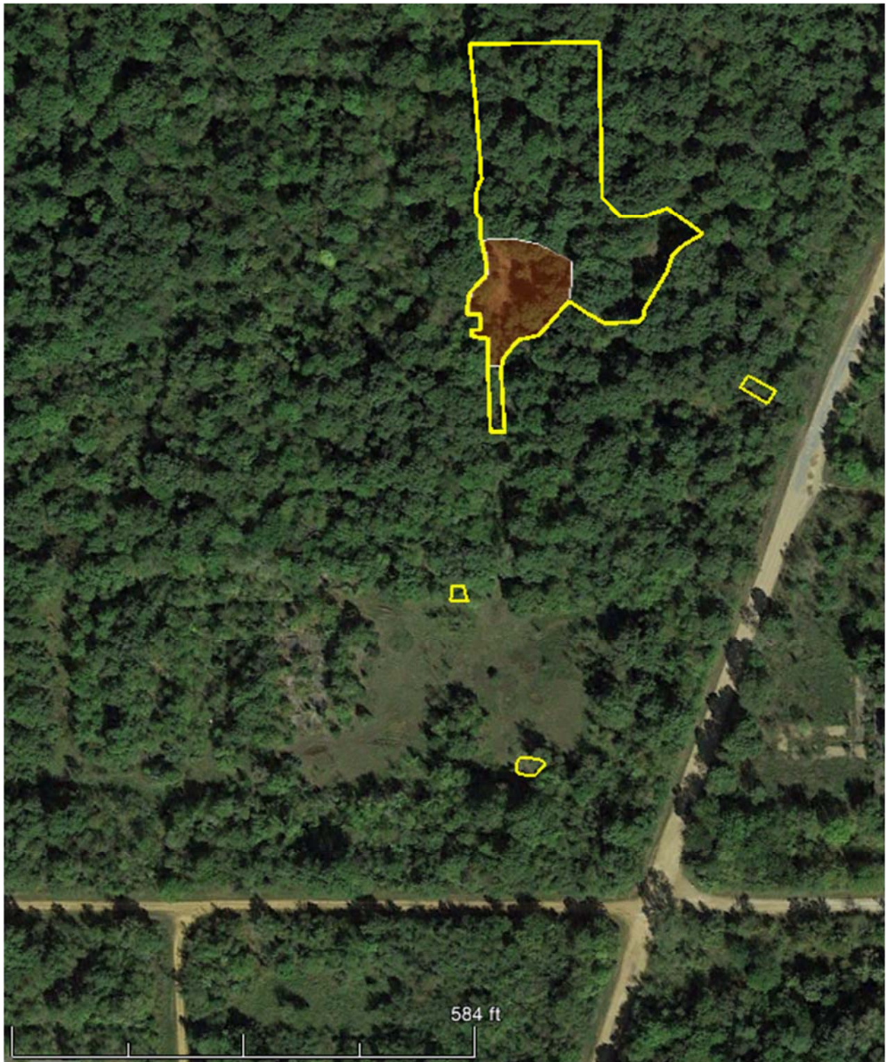
Yellow outlines indicate the contaminated areas. The brown shading indicates the area considered to be a hazardous waste.
