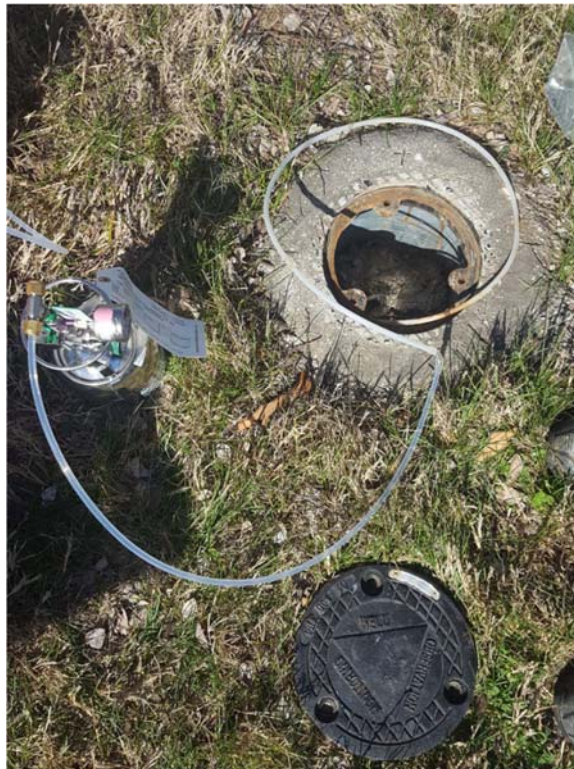
Vapor sample collected from a soil vapor probe. Summa canister (left) under vacuum that is used to extract soil vapor from probe via flexible tubing.
