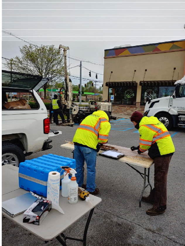
Wood personnel examining the soil cores as the drilling subcontractor works in the background.
